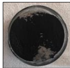
Figure 15:AC after surface modification
