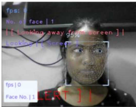
Fig.14 The alert is triggered as the gaze is away from the screen
