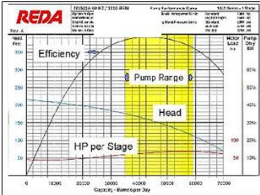
Figure 3. ESP Pump Performance Curve
