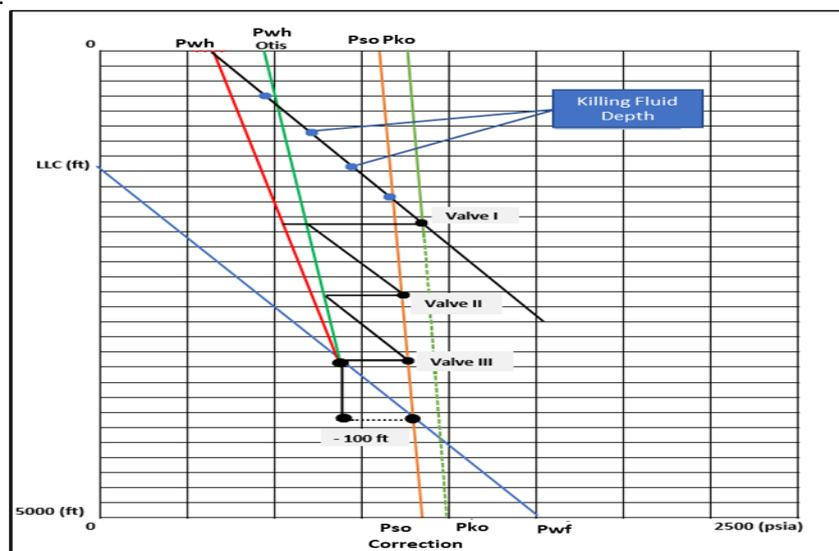
Figure 2. Gas lift design used Otis Method
