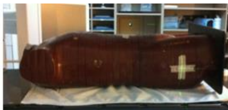
Figure 3. Rando phantom and OSLD inside the LINAC
