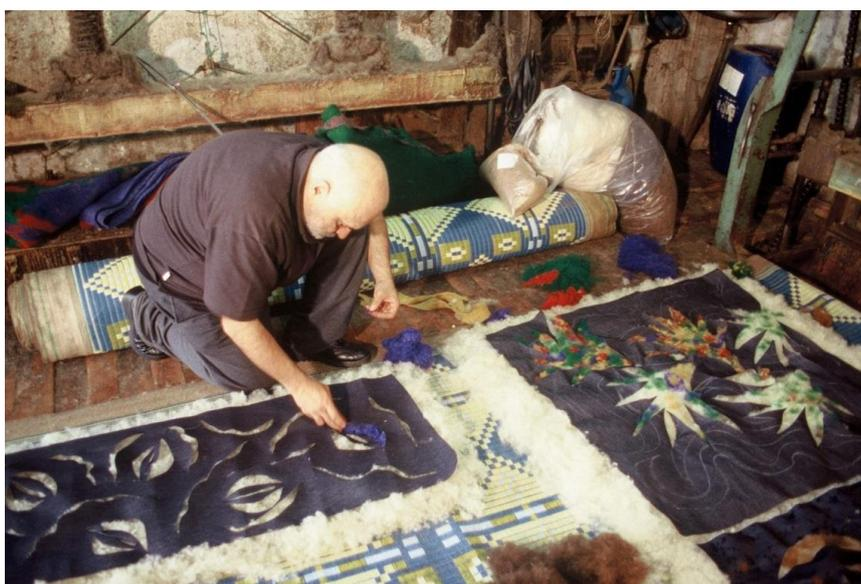
**Picture 8.** Conversion work by felting denim wastes and wool fiber together.
