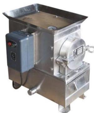
**Picture 7.** Small capacity (for sampling) textile and garment grinding/shredding machine.
