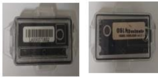
Figure 1. Optically stimulated luminescence dosimeter used in the experiment
