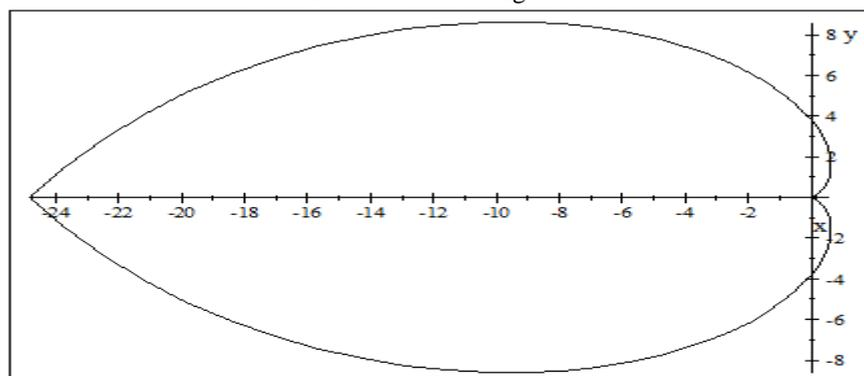
Figure 1: Region of Absolute Stability for Two-step with Off-step Point  $\frac{2}{3}$
