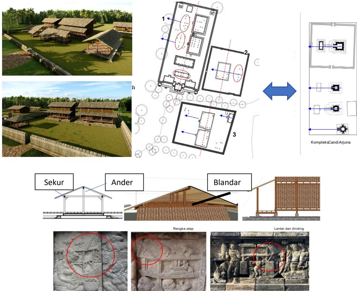
Fig 4. The Tectonic of Roof Construction, *Blandar*, *Ander*, *Sekur*[24]
