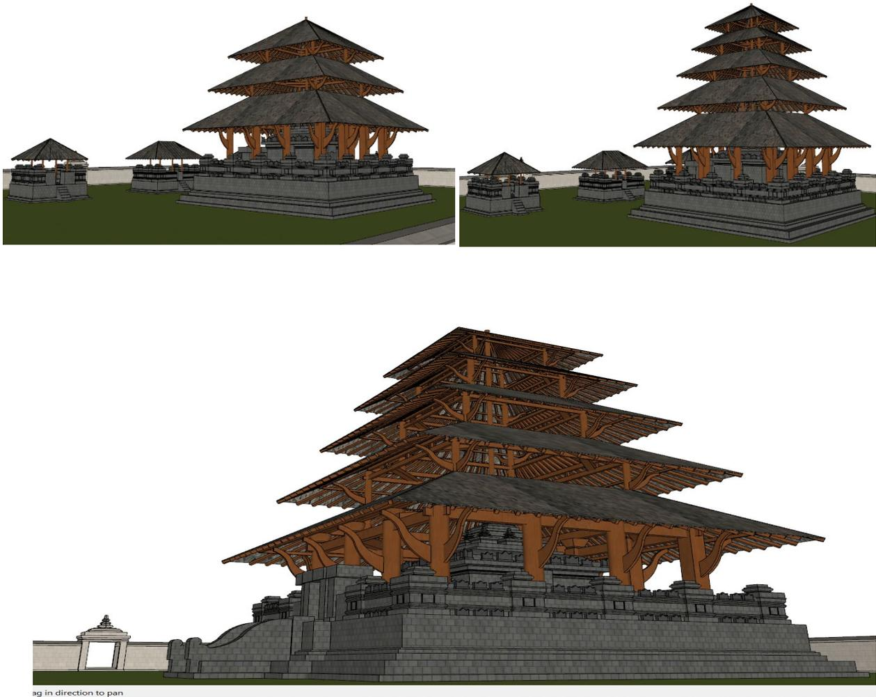
Fig 9. Upper : Ward off Rain Water, Cross Ventilation, Detail Wooden Construction; Below Column and Foundation (*umpak*) [24]
