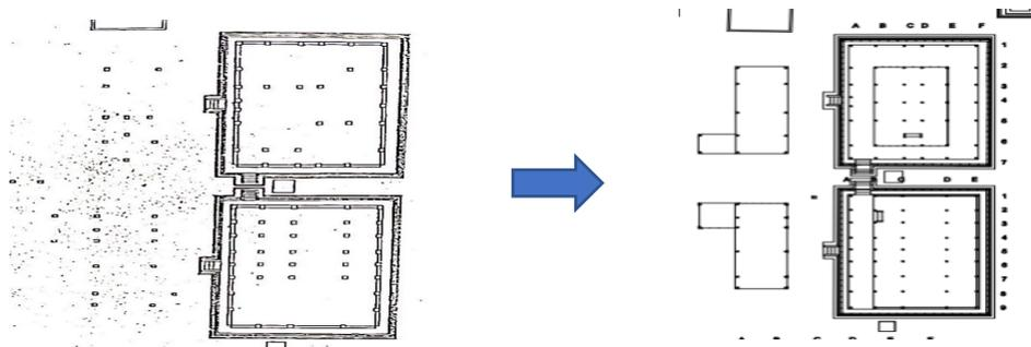
Fig 2. Reconstruction of column position [24]
