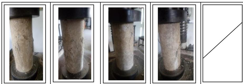
Fig 3. Cylinders type A at the age of 14 days have drawing sketch of type /shape of destruction on the specimen according to type 4 = shear destruction shape (SNI 1974:2011).<sup>[1]</sup>
