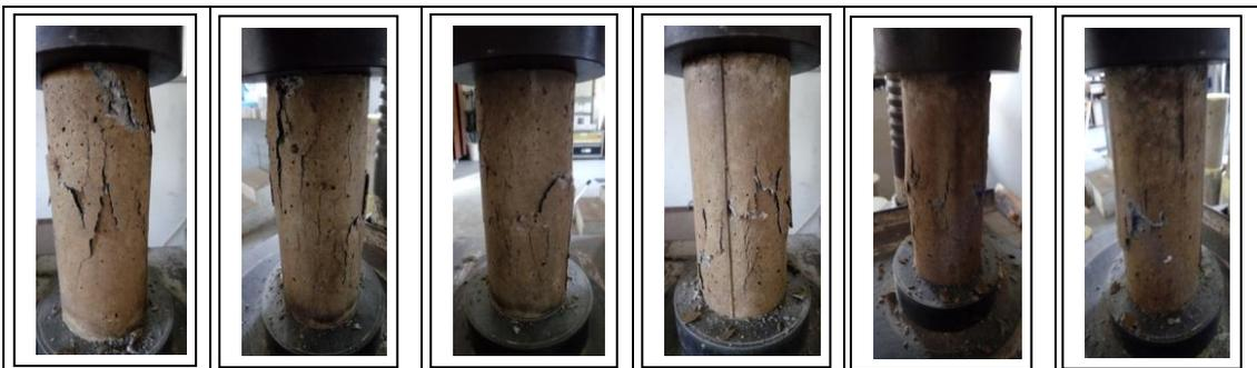
Fig 8. Cylinders type N /normal /without use bottle plastic /glass at the age of 28 days do not have drawing sketch of type /shape of destruction on the specimen according to SNI 1974:2011.<sup>[1]</sup> Cracks /breaks that occur do not have special pattern /irregular.
