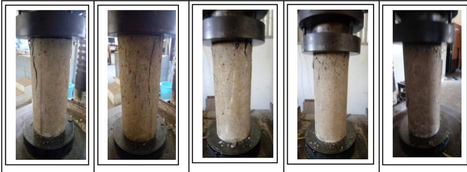
Fig 7. Cylinders type N /normal /without use bottle plastic /glass at the age of 14 days do not have drawing sketch of type /shape of destruction on the specimen according to SNI 1974:2011.<sup>[1]</sup> Only in the form of hair cracks /small cracks that do not have special pattern /irregular.
