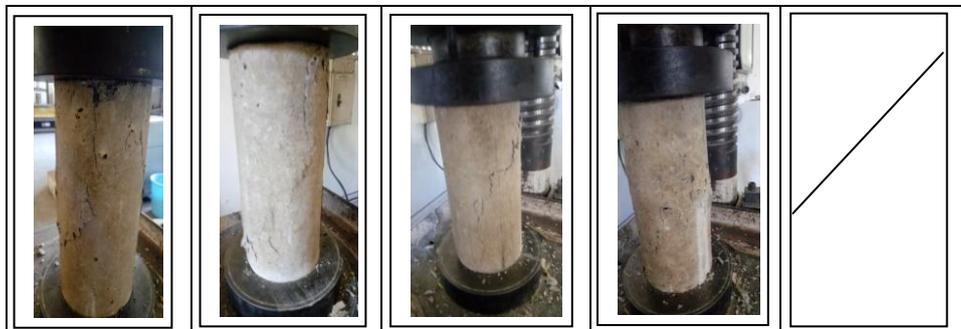
Fig 5. Cylinders type B at the age of 14 days have drawing sketch of type /shape of destruction on the specimen according to type 4 = shear destruction shape (SNI 1974:2011).<sup>[1]</sup>
