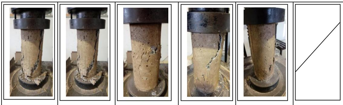
Fig 6. Cylinders type B at the age of 28 days have drawing sketch of type /shape of destruction on the specimen according to type 4 = shear destruction shape (SNI 1974:2011).<sup>[1]</sup>
