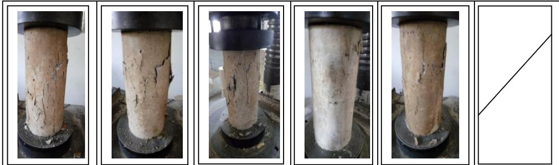
Fig 4. Cylinders type A at the age of 28 days have drawing sketch of type /shape of destruction on the specimen according to type 4 = shear destruction shape (SNI 1974:2011).<sup>[1]</sup>
