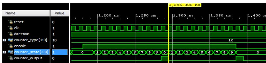
Figure 16. BCD counting up (original circuit)
