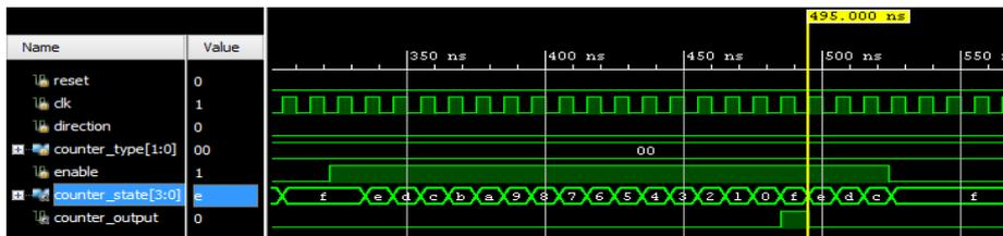
Figure 13. Binary counting down (original circuit)
