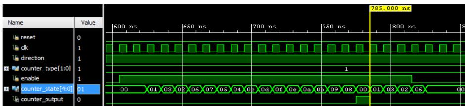
Figure 20. Gray code counting up (watermarked circuit)
