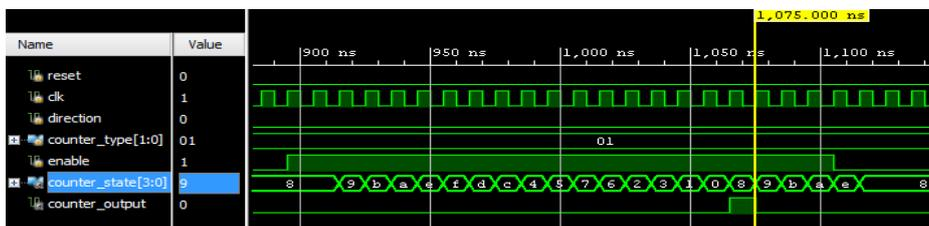
Figure 15. Gray code counting down (original circuit)
